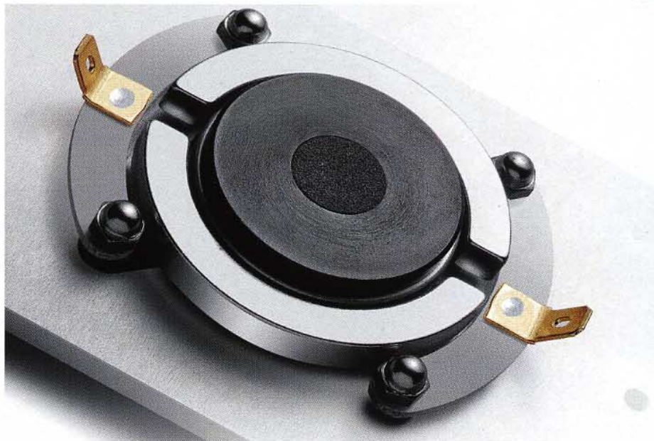
Rear view of beryllium-domed tweeter, showing two neodymium magnets enclosing the pole-piece, augmenting the main samarium cobalt magnet hidden within
